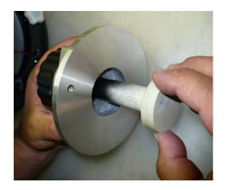
Install the encoder mount by applying a small amount of silicone glue to the top of the base and slide in the bearing assembly. Orient the threaded hole for the thumbscrew to the right. This is looking from the outside while holding the bearing assembly with it's curved end down. Allow the silicone to cure for 12-24 hours.
