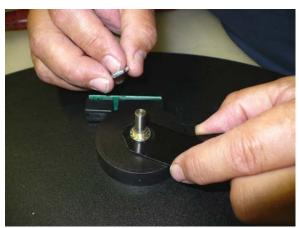
Press the encoder shaft into the Tension Knob and tighten the pivot bolt setscrew with the supplied 5/64" hex key.
