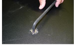
Install the 3/8" T nut into the groundboard from the bottom (foot side) using a scrap piece of wood while tapping in with a hammer so the T nut is not deformed.
