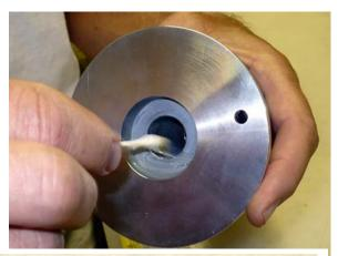
Remove the nut and one star washer from the altitude encoder and place the tangent arm on the encoder. Replace the outer star washer, thread the nut on the
