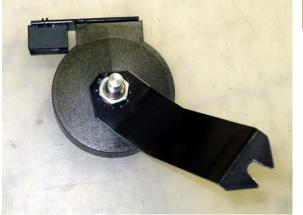
encoder. Orient the tangent arm as in the photo and tighten the nut.
