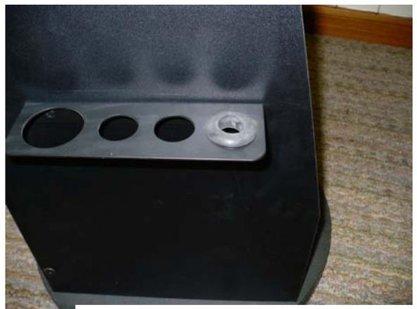
Slide the Computer mount post through the grommet in the eyepiece rack and align vertical by checking from the front and side. Mark around the outside of the truss and remove. Find the center of this circle and using a 1/8" drill bit drill 5/8" deep. Install a #8 x 3/4" screw through the tube retainer and install in the
