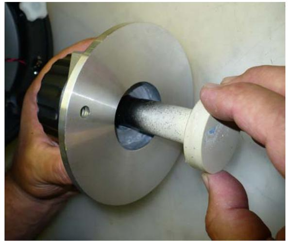
Install the encoder mount by applying a small amount of silicone glue to the top of the base and slide in the bearing assembly. Orient the threaded hole for the thumbscrew to the right. This is looking from the outside while holding the bearing assembly with its curved end down. Allow the silicone to cure for 12-24 hours.
