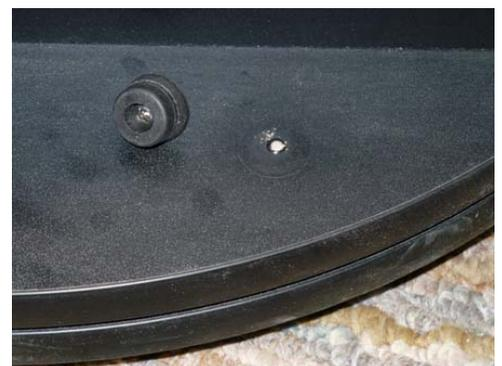
rocker box. The photo shows the tube retainer with screw next to it's mount hole. Slide the mount post through the grommet and onto the tube retainer.
