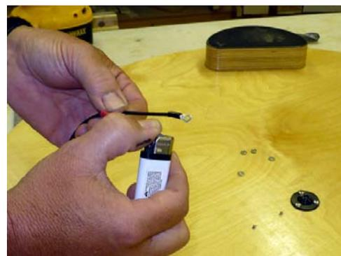
Strip about 3/8" of the insulation from the grooved (+) side, insert into the red insulated connector and crimp the connector. Attach to the screw by first placing a washer over the screw, then the connector and a nut.
