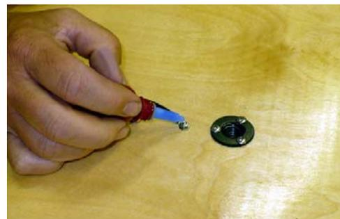
Apply Loctite or fingernail polish and tighten the nut. Cut the smooth wire to length to match the un-insulated connector at the screw from the smaller ring (-). Slide the provided heat shrink insulation on the wire, and crimp the connector. Slide the heat shrink onto the connector and using a lighter or match, shrink the insulation (see photo at right). Place a washer on the screw, then the connector(-) and a nut, tighten using Loctite or fingernail polish to secure the nut.
